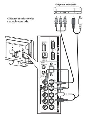
3 Connect an audio cable (included) to the COMPONENT IN L/R audio jacks on the back of your TV and to the L/R AUDIO OUT jacks on the component video device.
